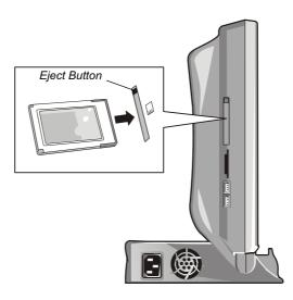
3. When a PC card is seated, the computer will detect it and try to install the appropriate driver. Follow the on-screen instructions to complete the process.
