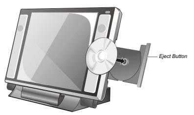
To remove a CD, slightly press the center of the CD and, holding the CD by its outer edge, lift it away from the tray.
