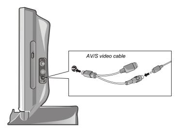
**If you are connecting an S-video device:** Plug the cable from the device to the S-video connector on the AV/S video cable.
