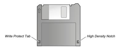
The drive is a high-density 3.5-inch one, which can read and write to either double-density (2DD) 720-KB floppy disks or high-density (2HD) 1.44-MB floppy disks. A floppy disk have an arrow imprinted on the front upper left corner, and a sliding write-protect tab on the bottom left corner, as illustrated above. When opened, the write-protect tab prevents data from being written to or erased from the floppy disk.
